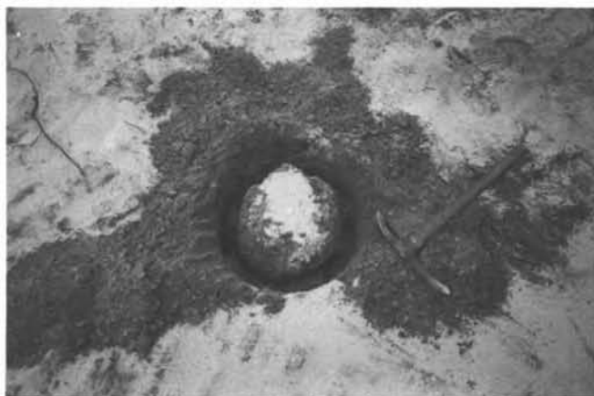
FIG. 1. Circular trench and trenching tool.
